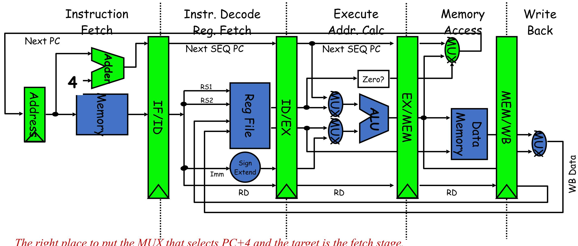
The right place to put the MUX that selects PC+4 and the target is the fetch stage.
